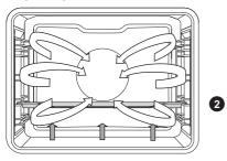
This is used for baking leavened but lowrising pastry and for preserving fruit and vegetables. Use the second guide from the bottom and a rather shallow baking tray to allow the hot air to circulate across the upper side of the dish.
