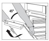
**3** Slowly close the door to a 45-degree angle (relative to the position of the fully closed door); then, lift the door and pull it out.
