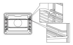
The grid or the tray should always be inserted into the groove between the two wire profiles.
