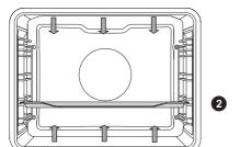
The heaters in the bottom and in the ceiling of the oven cavity will radiate heat evenly into the oven interior.
