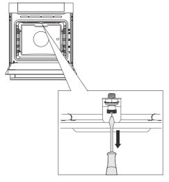
**1** To remove the heater, undo the screw located at the front of the oven cavity ceiling.
