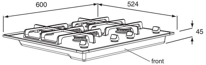
Minimum distance between rear of appliance and rear wall: 10 mm
