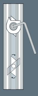
Insert into post channel and slide to desired height. Level shelf by adjusting shelf peg positions and tighten screw using hex key.
