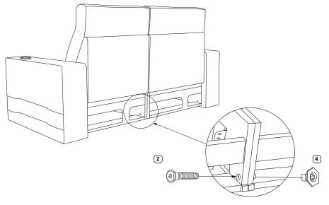
**B.** Remove lower back panel and locate the back bolt holes.
