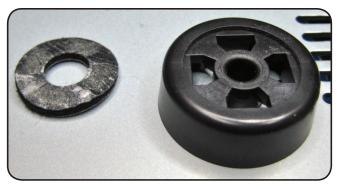
4. Identify the four locking tabs securing the foot to the chassis. The photo of a removed foot shows the details of the locking tabs.
